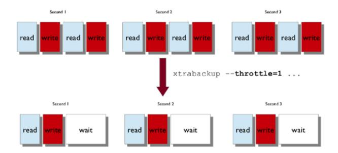
In —backup mode, this option limits the number of pairs of read-and-write operations per second that xtrabackup will perform. If you are creating an incremental backup, then the limit is the number of read IO operations per second.
